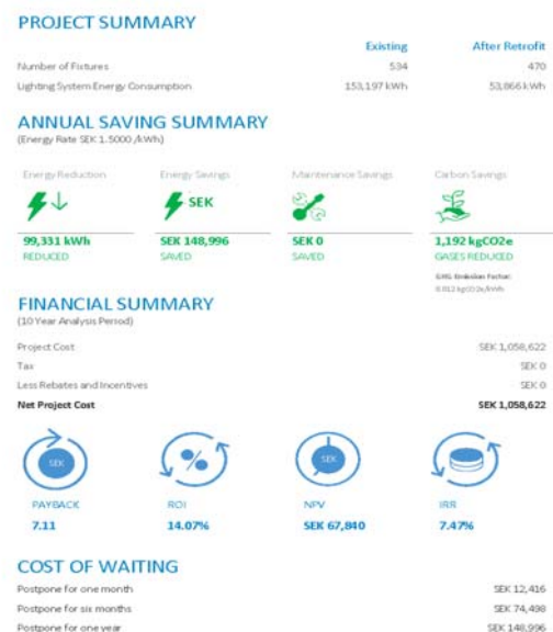
Figure 12. A brief summary of the project for the main building of SSSL
