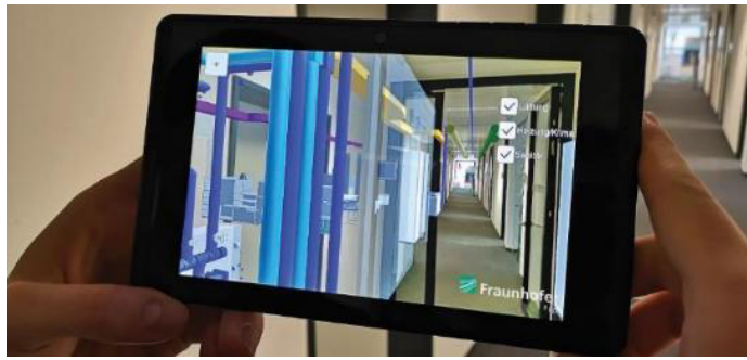
Figure 11. BIM-enabled mobile mixed reality visualisation of heating and ventilation pipes in the Ellinogermaniki Agogi building (Source: Doerner et al, 2019 18 )
